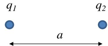
$$\vec{E}(\vec{r}) = \frac{1}{4\pi\epsilon_0} \left[ \frac{q_1 (\vec{r} - \vec{r}'_1)}{|\vec{r} - \vec{r}'_1|^3} + \frac{q_2 (\vec{r} - \vec{r}'_2)}{|\vec{r} - \vec{r}'_2|^3} \right] \quad (1)$$
